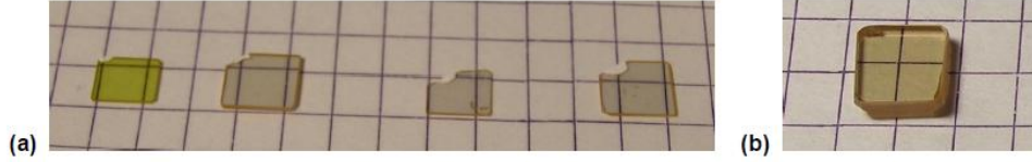
Fig. 4. (a) AGS (left) and 3 BGS samples used for determination of the nonlinear coefficients, and (b) BGS damage test plate.
