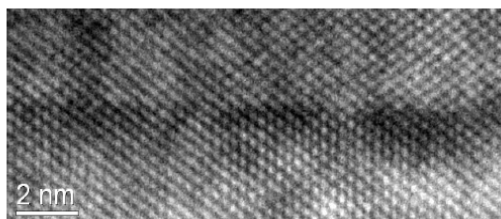
Figure 5 TEM view of domain wall, where one observes the continuity between the crystallographic plans between the two domain orientations.
