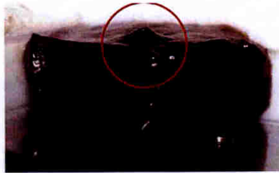
Fig. 2: Picture of a liver tissue sample after ablation using the CSP-based SPOPO.
