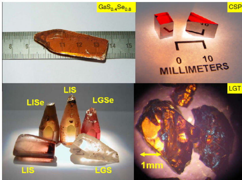
Fig. 4. Layered crystal of \text{GaS}_{0.4}\text{Se}_{0.6} : the maximum S-content preserving the noncentrosymmetric structure of the mixed compound (the transmission in the visible is obviously improved in comparison with GaSe), cube and prism made of CSP to measure thermo-mechanical and dispersive properties, ingots of orthorhombic Li-compounds after annealing, and first grown samples of LGT [courtesy of V. Panyutin (Kuban State University), top-left, P. Schunemann (BAE Systems), top-right, and L. Isaenko and A. Yelisseyev (Institute of Geology and Mineralogy), bottom pictures].
