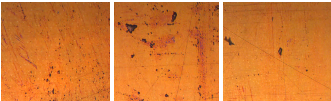
Fig. 8 Microscope pictures of surface segments of one of the uncoated test plates of LISe before the damage tests (size of the above pictures is appr. 2 \text{ mm} \times 2 \text{ mm} ).
