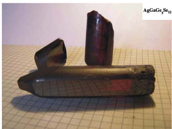
Fig. 1. Photograph of single crystals of AgGaGe_5Se_{12} : The front boule has a size of \phi = 18 \times 80 mm.
